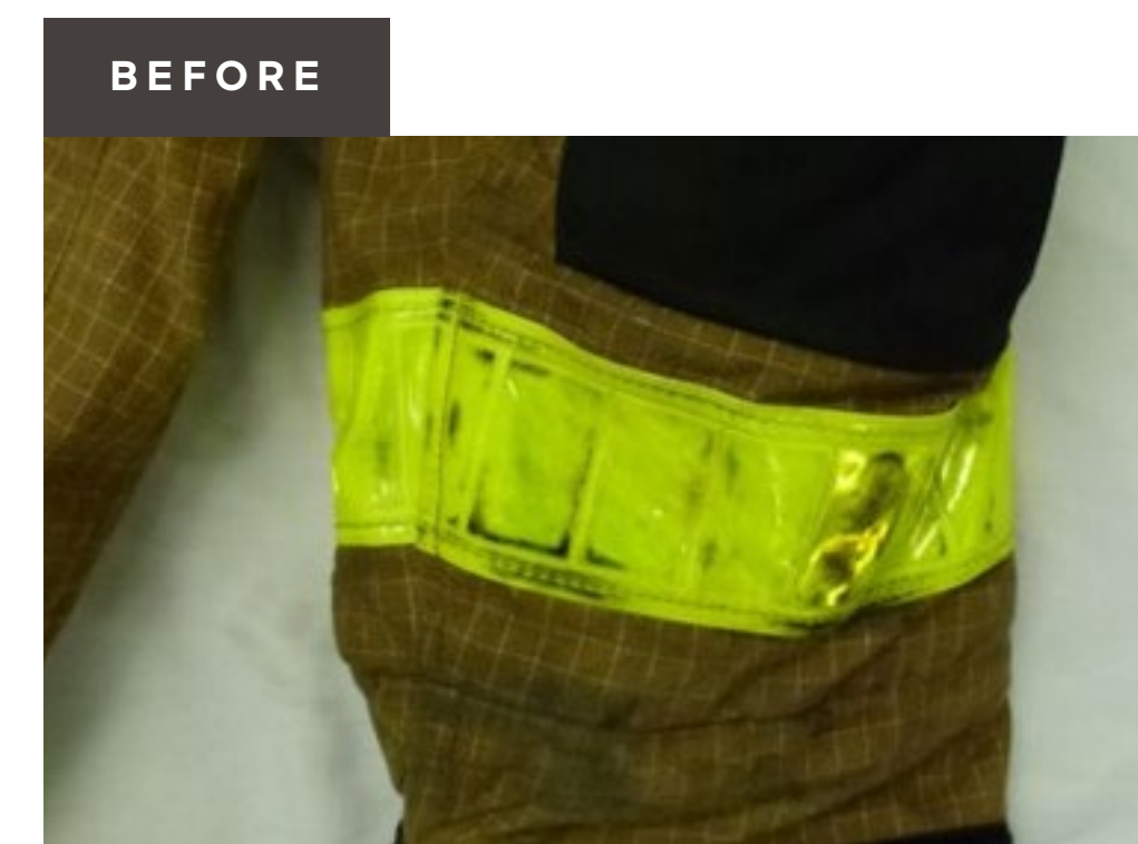
Condition of jacket prior to tests – note the level of soiling on the arms.
